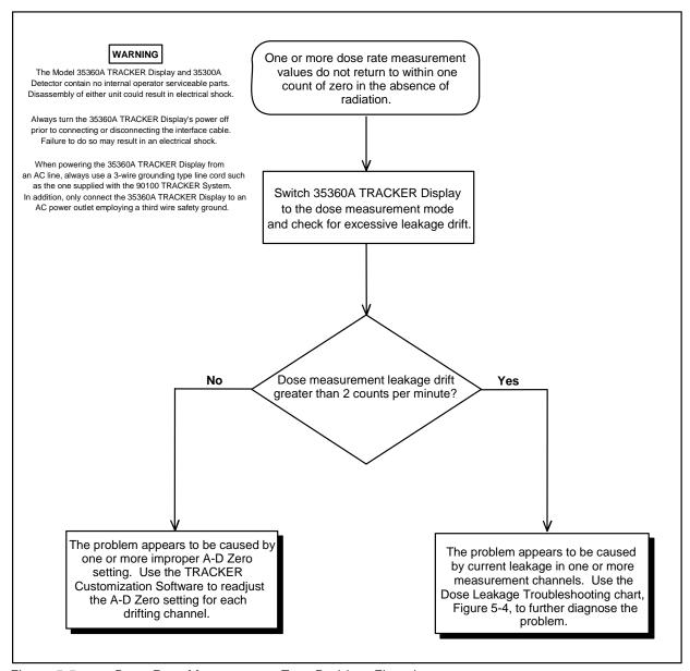
Figure 5-5 Dose Rate Measurement Zero Problem Flowchart
